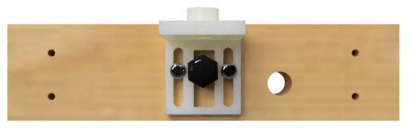
**Secure with 6mm x 100mm Screw:** Insert the long 6mm x 100mm screw through the center hole of the bracket and into the corresponding hole in the wood. Add a nut to the the screw to hold it firmly in position.
